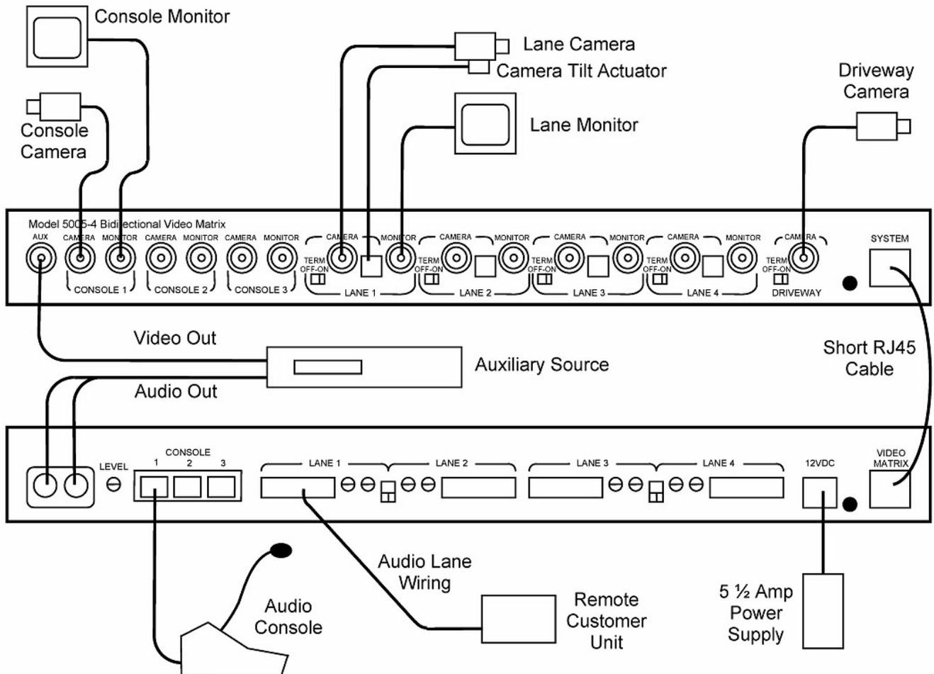
1. Remove power from the 5002 audio matrix. Connect the short RJ-45 cable supplied with the video matrix between the video and audio matrixes (n/a for model 5006).
