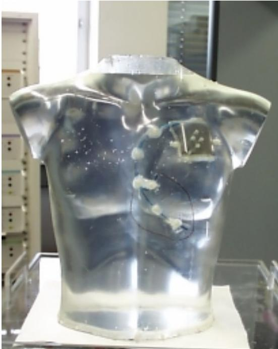
**Figure 15:** Phantom with implanted ICD
