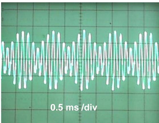
**Figure 2.:** Wave form (time domain) of the magnetic field emitted by the 02PN10
