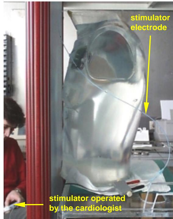
**Figure 12:** Phantom in worst case exposure situation during the stimulation test
