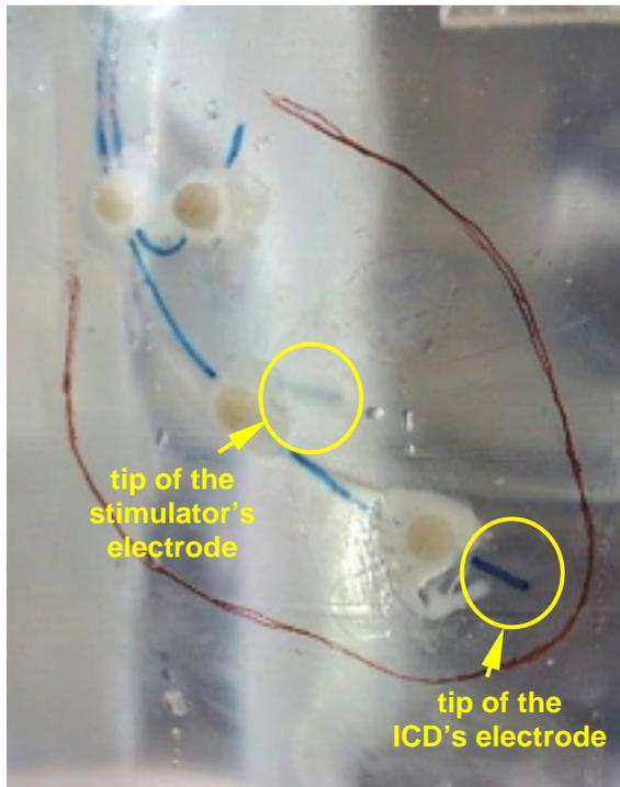
**Figure 11:** Location of the stimulator's and the ICD's electrodes
