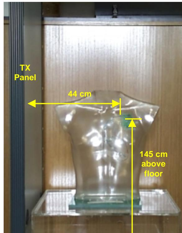
**Figure 9:** Exposure Situation D. Standing in the centre of the Metal Detector Gate, the implant closer to receiving panel
