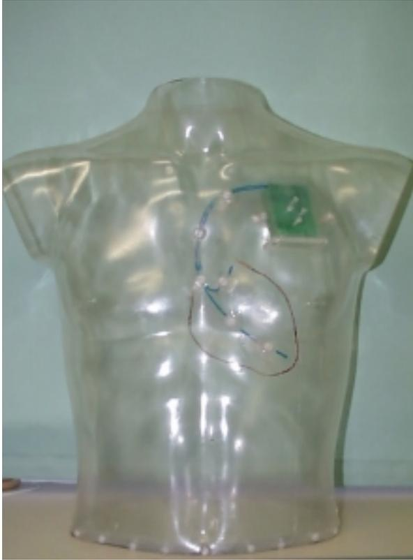
**Figure 13:** Front view of the phantom. The approximate outline of the heart (red) and the positions of the electrodes (blue) are drawn on the phantom's surface. In the upper left breast region an ICD-dummy (green coloured) is mounted according to the left-pectoral implantation method. The mounting for the ICD is designed in a way to allow a liquid layer of about 1 cm between the implant and the phantom shell to reflect the corresponding tissue layer.
