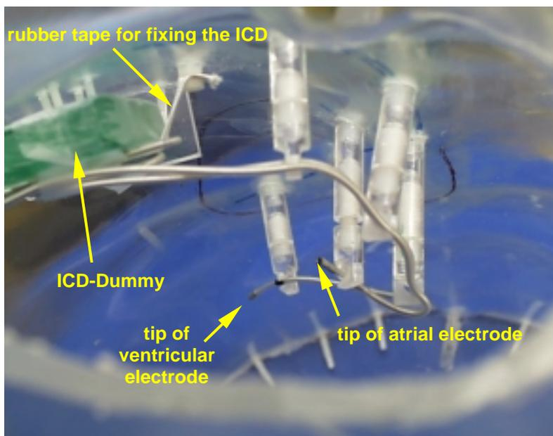
**Figure 14:** View from the top back into the neck of the phantom. The ICD-dummy is fixed in its fixture by a rubber tape. The atrial and ventricular electrodes are fixed in special mounting pins reflecting the conditions of a two chamber ICD. The electrodes on the photograph are not applicable to ICDs. They are used for demonstration only in this figure.
