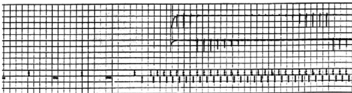
Cut-out of the stimulation test during exposure. At the left side (before stimulation) the ICD is pacing properly. After set-in of the stimulation the ICD detected the fibrillation correctly.
