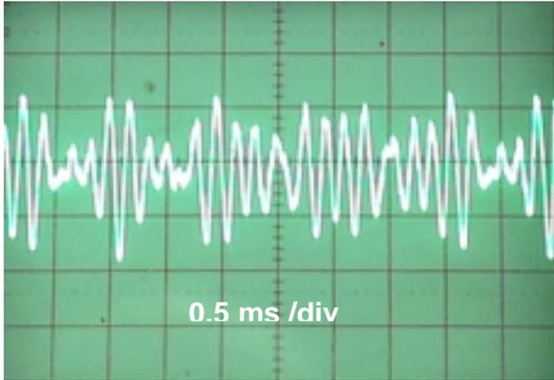
**Figure 5:** Wave form (time domain) of the magnetic field emitted by the PMD2/PTZ
