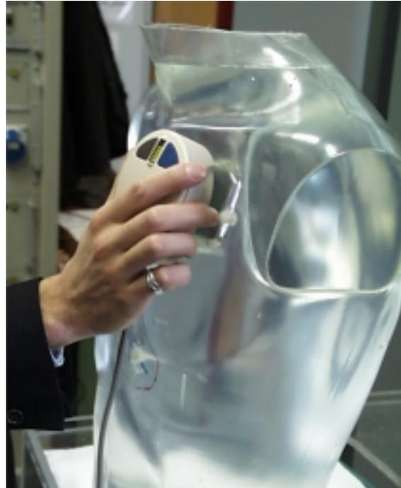
**Figure 16:** Phantom during the read out of the ICD's event storage
