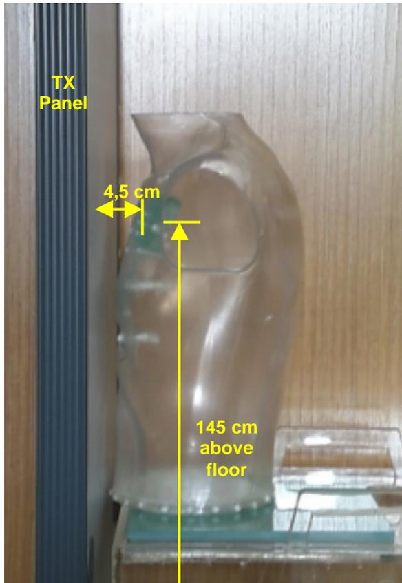
**Figure 10:** Exposure Situation E. Standing in front of the transmitting panel with the breast as close as possible to the panel
