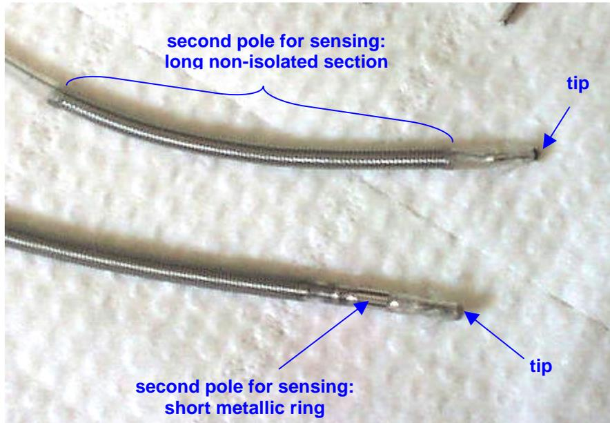
**Figure 17:** Lead sections of one 'integrated bipolar' (top) and one 'true bipolar' (bottom) electrode type.
