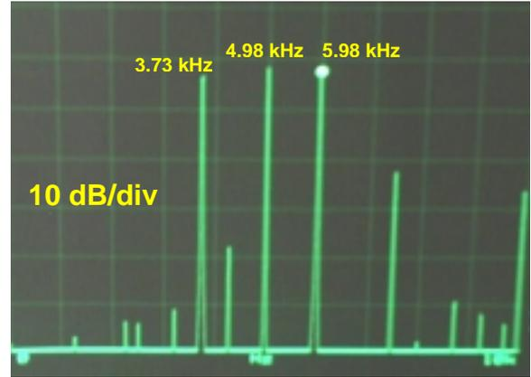
**Figure 6:** Frequency spectrum of the magnetic field emitted by the PMD2/PTZ
