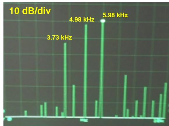
**Figure 3.:** Frequency spectrum of the magnetic field emitted by the 02PN10
