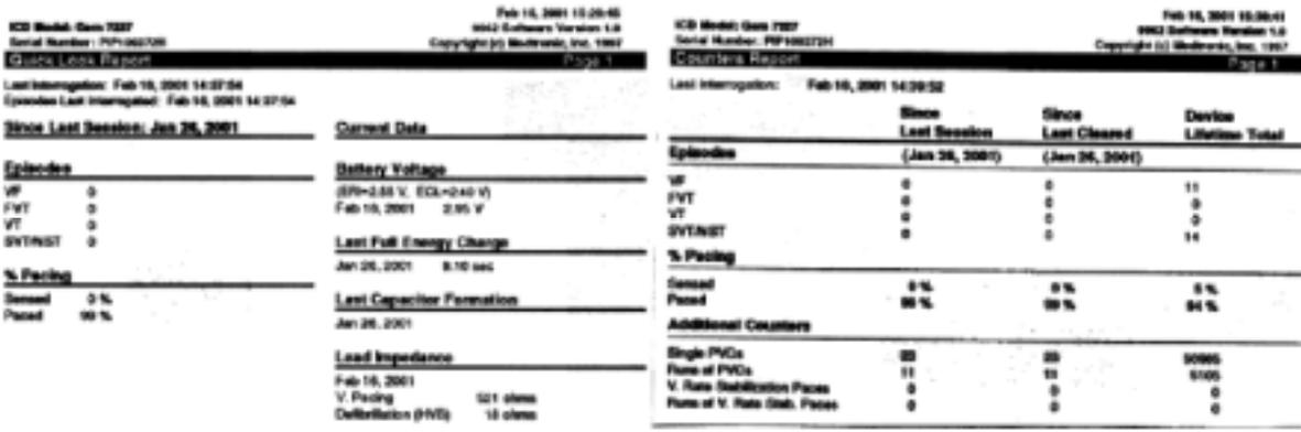
Event counter status before (left page) and after (right page) exposure to the metal detector systems. The event counter hold the same values before and after exposure, i.e. no episodes are falsely sensed during exposure.
