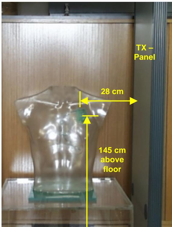
**Figure 8:** Exposure Situation B. Standing in the centre of the Metal Detector Gate, the implant closer to transmitting panel
