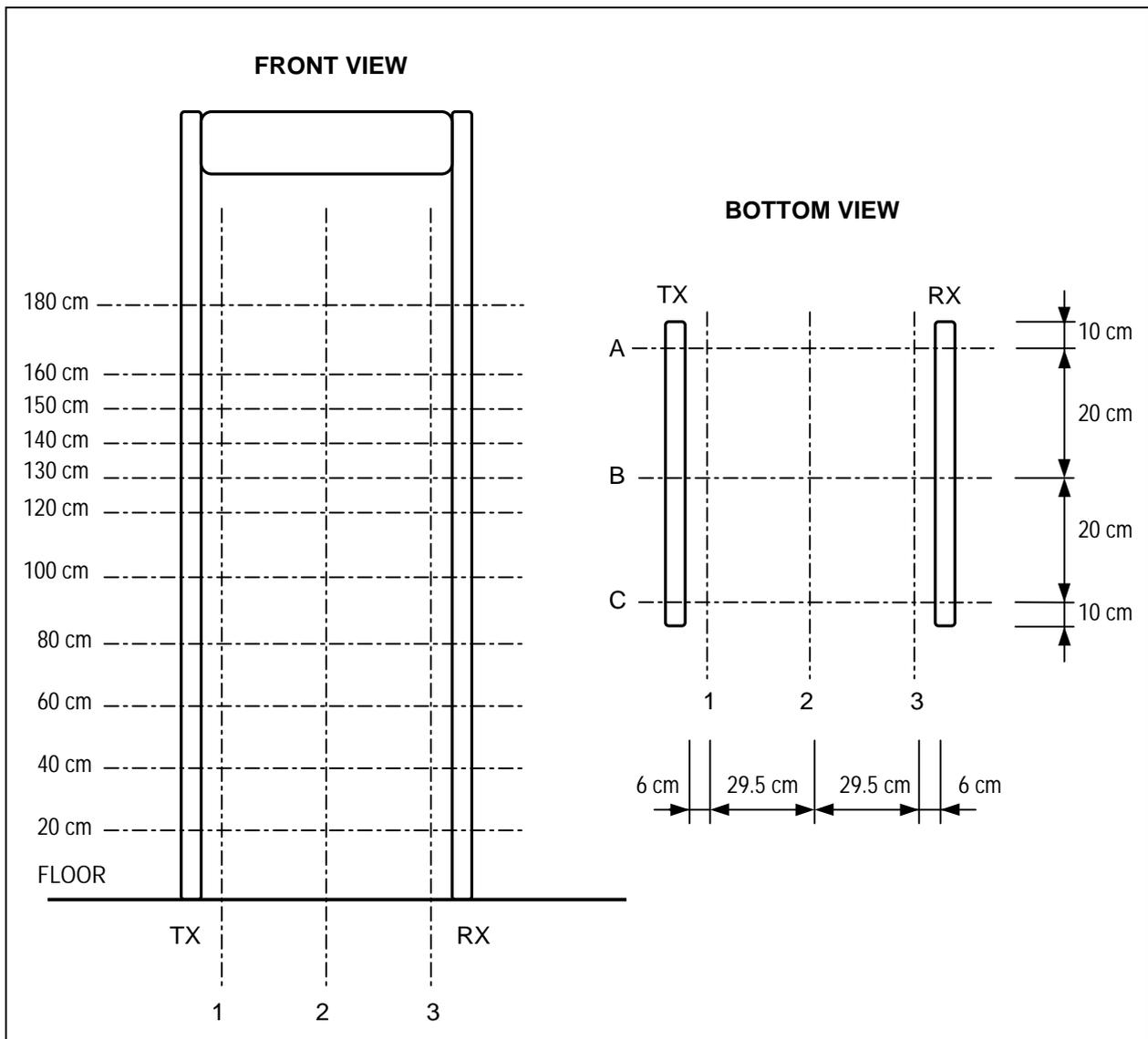
**Figure A.1:** Definition of measurement grid for the measurements of magnetic induction.
