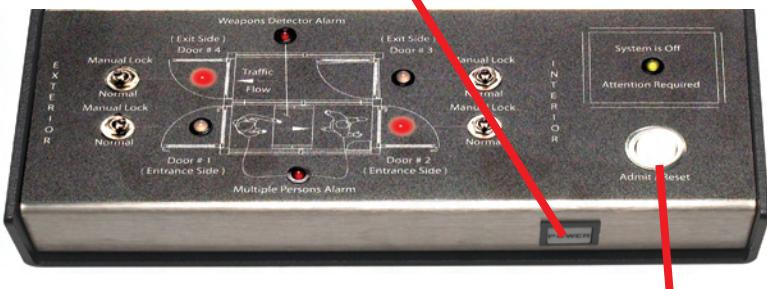
3. Be sure that **all Door Locking Control Switches** (#11) are in the down position; that is, pointed towards the bottom of the Operators Console as shown above.
